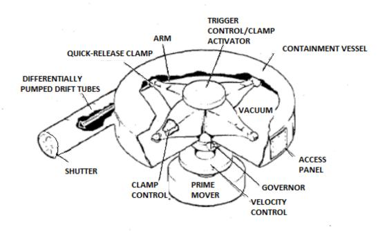
Figure2: Edge-release centrifugal projectile accelerator
