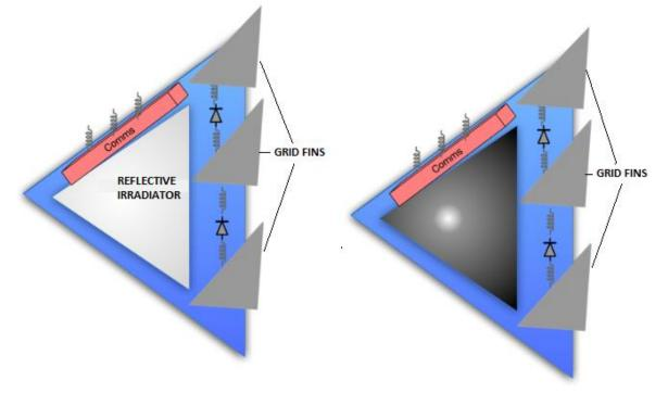
Figure3: Micro-bot with reflectivity control
